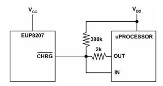
Figure 5. Microprocessor Interface
