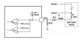
Figure 7. Temperature Sensing Thresholds
