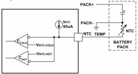
**Figure 6. Temperature Sensing Configuration**
