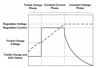
Figure 4. Typical Charge Profile
