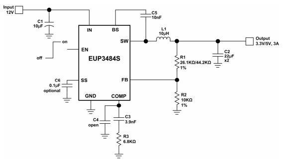
Figure 1. 12V to 3.3V/5V Application Circuit
