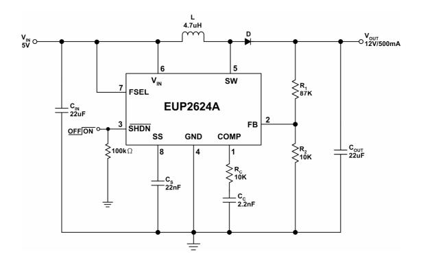
Figure 1. 5V to 12V Step-Up
