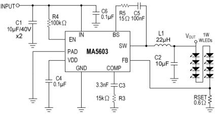
$I_{LED}=V_{FB}$  /RSET=0.2V/0.6 $\Omega$ =0.330A ,  $V_{FB}$  = 0.2V.
