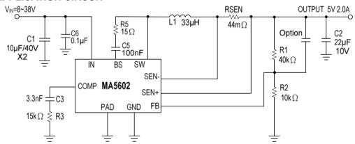
$V_{OUT} = V_{FB} \times (1 + R1/R2), V_{FB} = 1.00V, R2 \text{ suggest } 10k \sim 30K\Omega$  $I_{SEN} = V_{SET} / RSEN = 100mV / 44m\Omega = 2.27A$
